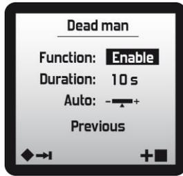
**Duration:** time in seconds before a shutdown is triggered if no control system has been activated or if the inclinometer has not detected any movement. By default, a pre-alarm is triggered 5 seconds before shutdown is triggered\*.
