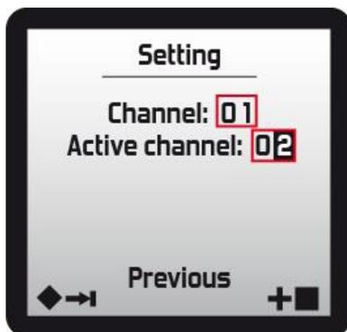
**Rest channel:** all receiver modules in the group are in listening mode on this channel until start of operation.
