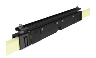
Air Gaps are used for the galvanic isolation of sections, such as maintenance segments that can be supplied with power and turned off separately. For each separation point, two Air Gaps must be mounted at a suitable distance to avoid power carryover through the Current Collectors.
