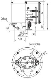
Bore holes in the floor panel intended for the following screw connections: 1x M63x1.5, 1x M40x1.5, 1x M32x1.5
