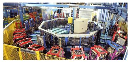
Rotary injection-molding machine from Krauss-Maffei Kunststofftechnik (Munich)
