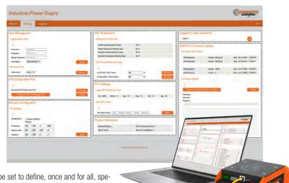
and voltage requests provided. Manual parameters can also be set to define, once and for all, specific current and voltage requests to follow. This specific mode operation is possible even without communication links to the battery or vehicle control unit. All those important parameters are set thanks to an embedded Webserver hosted inside the electronics unit i.e. the MPU.
