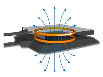
radio waves as occurring in radio communication or with mobile phones: these are electro-magnetic waves designed to be sent out to bridge large distances. It must also be noticed that magnetic fields, as used in **WirelessCharger 3.0** as means for power transfer, are linked to their source, so they are always limited to the very proximity of the pads.
