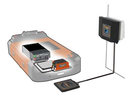
Applying **opportunity charging** implemented in operation processes allows typically smaller batteries and increases the lifetime of batteries by the means of short but more frequent charging sessions the lifetime of batteries, as this method of charging results in less thermal stress in the battery.
