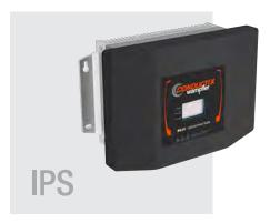
The **IPS** (Inductive Power Supply), converts the 50 or 60 Hz mains frequency into a high frequency allowing highly efficient power transfer. Charging requirements and other information coming from the Battery management system onboard the vehicle is taken up by the ISP and transferred in corresponding action.
